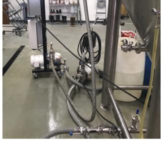
**LEFT: The** ShockWave Xtractor takes up a small footprint and is placed on casters so that the brewers at Cabarrus Brewing Company can easily move it around to different tanks in the brewhouse. Photo courtesy of Cabarrus Brewing Company.
