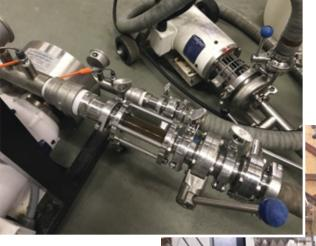
ABOVE: Cabarrus Brewing Company uses the ShockWave Xtractor from Hydro Dynamics, Inc. to extract more flavor from hops and speed up the brewing process. Photo courtesy of Cabarrus Brewing Company.
